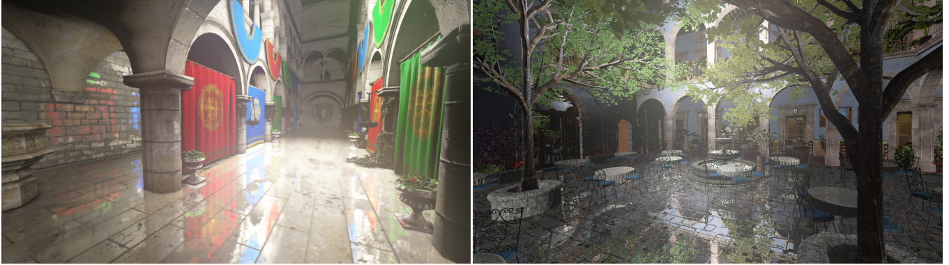
Figure 1: With our hierarchical multi-layer ray tracer, advanced effects, especially from long rays, can be rendered efficiently. Both images shown demonstrate two-bounce screen-space reflections. Note the reflection of the red and blue curtains in the left-most part in Sponza and the reflections in the windows of San Miguel. Render times for multi-layer framebuffer generation are 1.34 ms, computing our hierarchy takes 1.98 ms and tracing two reflections bounces 4.93 ms (left), and render 5.62 ms, hierarchy 2.09 ms and tracing two bounces 5.25 ms (right). All at 720p with 4 layers on Geforce 1070 GTX without any further common optimizations such as sub-sampling or increased strides.
