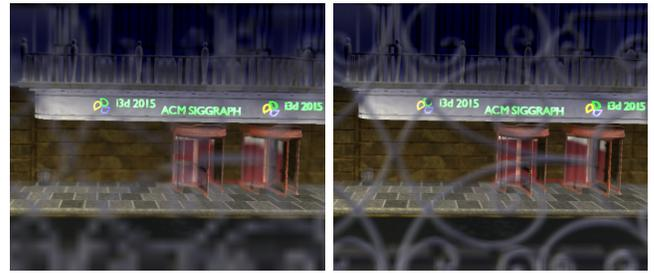
**Figure 3:** Filtering multiple levels using the mip-mapping scheme only exhibits strong artifacts, especially for the near field (left). The use of a filter stack preserves the fine structure while still filtering it appropriately (right).
